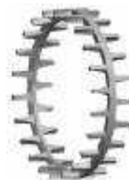
Fig. 6. EMB/YMB One-piece, machined-brass, land-riding, finger-type cage.
