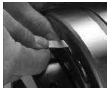
Fig. 18. Measure RIC before installation.
