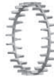
Fig. 45. One-piece, machined-brass, land-riding, finger-type cage.
