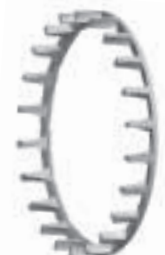
Fig. 46. Split, machined-brass, land-riding, finger-type cage.
