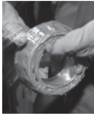
Fig. 147. Grease can easily be packed by hand.
