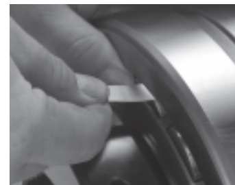
Fig. 95. Measure of RIC before installation.
