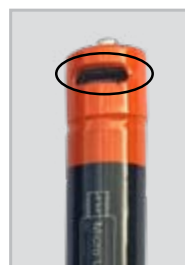
Li-ion Battery with in-built micro USB port
