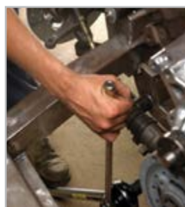
Torque multiplier used in inaccessible areas
