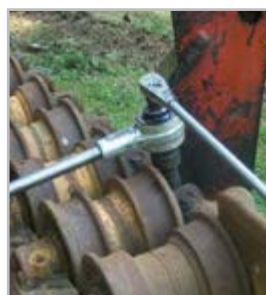
Torque multiplier used on tracks
