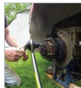
Torque multiplier used for lug nuts
