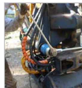
Torque multiplier used for machine nut tightening
