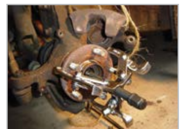
3 Jaw Puller used for removing tyre hub
